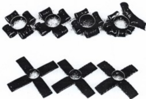
Fig. 4. Tube splitting due to axial loading [47].
