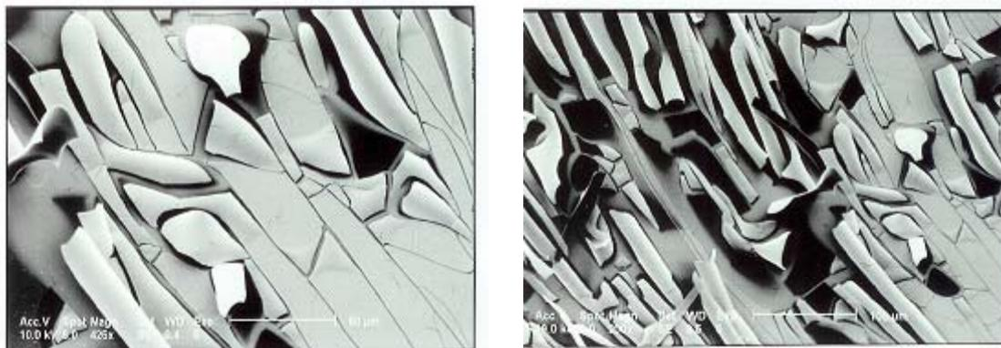
**Fig. 4: Scanning electron micrographs of Ni<sub>89</sub>P<sub>11</sub> glassy alloy at different magnifications in 3.0 M HCl solution.**
